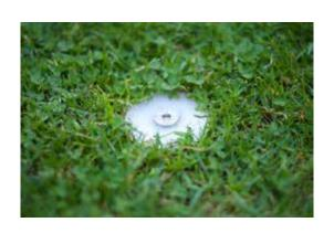
20 mm square rod, 300mm long tapered at one end M8 tap at other end to 30mm deep
